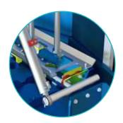
Automatic wire binder of drill type and seprate wire cutter
