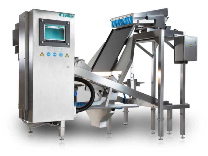
Designed with only PET processors in mind - the SORTEX E PolyVision<sup>™</sup> is Bühler's all-new optical sorter for polymer contaminant removal, complementing the existing PET flake sorting portfolio.
